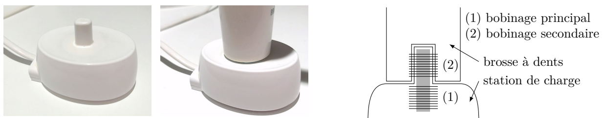
Figure 9 Station de charge
